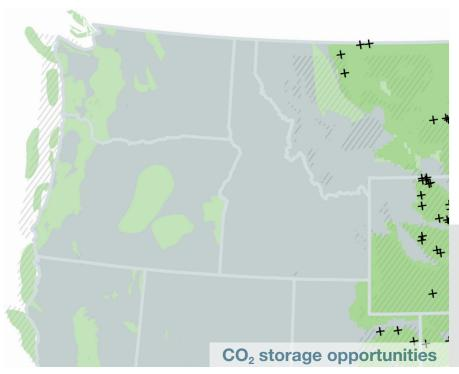
The Pacific Northwest has potential to act as a carbon storage destination for capture facilities and carbon removal. The states of Washington and Oregon have the combined potential to store 214 billion metric tons of CO<sub>2</sub> in secure geologic saline formations, and also have capacity for carbon storage in geologic fossil basins.
